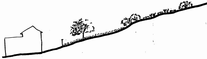
Section- Typical Fuel Break with Downhill Housing
